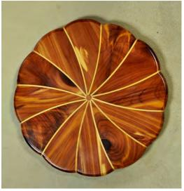
Note the darker and lighter separation pieces were cut using the same jig as the individual spiral pieces.
